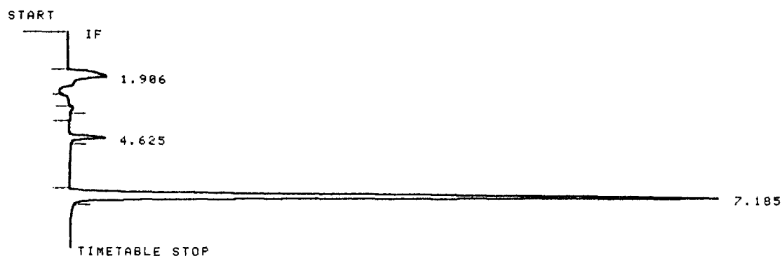
Fig. 6. Chromatogram of Bisalax micro-enema sample showing bisacodyl monoester at 4.6 min.
